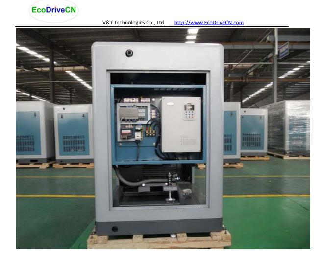
V/F control & vector control AC frequency inverters for air compressors
