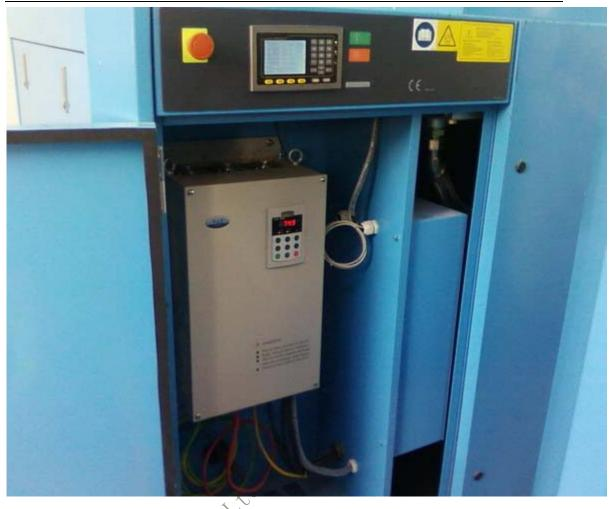
variable frequency AC inverter applied on air compressor for energy saving ud or. V&I Technologies
